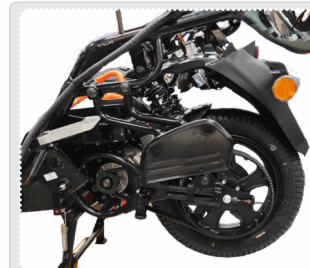
Mid mount motor with belt drive
